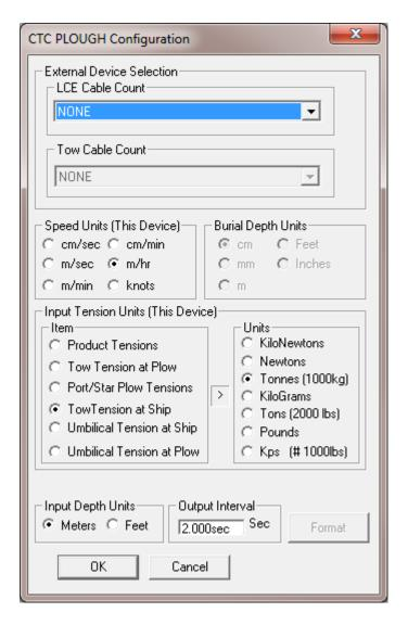
In the External Device Selection section, select the LCE Cable Count source from the dropdown list. Configure the Input Speed Units, Input Tension Items and related Units as well as the Input Depth Units.
