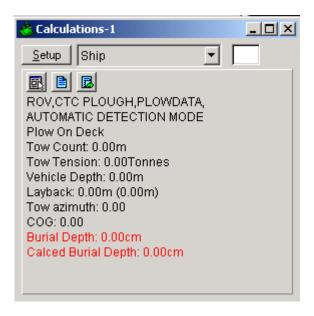
From this window, you can monitor some of the input data as well as the layback calculation. This Calculation window also provides a shortcut to the Configure Plow dialog box by clicking the button.
